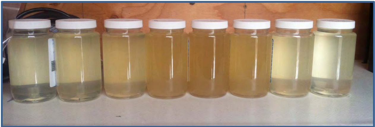
Figure 1: Water samples collected at 2 hour intervals (over a 48 hour period) with the ISCO sampler on Shashawandah Creek. This photo captures the change in suspended sediment in the creek throughout a storm event in March. As the water levels in Shashawandah rose, the waters became more cloudy with suspended sediment and when the water receded, the samples began to clear again.
