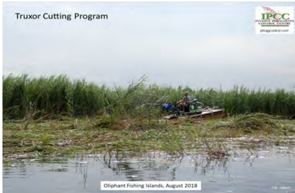
Figure 10. Truxor cutting high density Phragmites in a Lake Huron coastal wetland.
