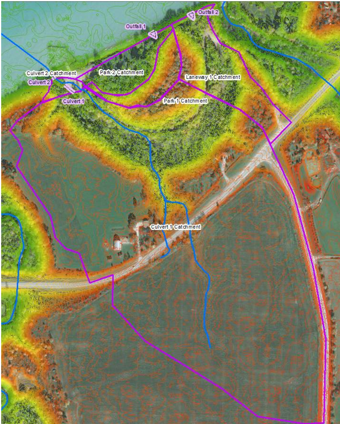
Figure 12. Catchment Areas and Outfalls
