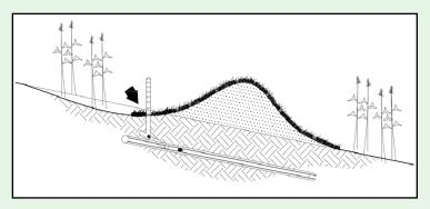
Narrow based berms are permanently vegetated, crops can be grown on either side.
