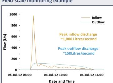
In the above example, it was found that WASCoBs reduced the magnitude of peak flow by about 85%. The duration of outflow was also increased from less than 1.5 hours to 9 hours with the installation of the WASCOB, a time period that won't cause flood damage to crops. Graph courtesy of Ausable Bayfield Conservation Authority.
