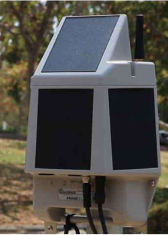
The Advanced Warning Equipment (AWARE) Flood System by AWARE Monitoring Systems.
